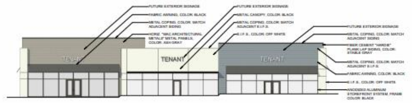
1 ELEVATION BUILDING G - EAST 3/32" = 1'-0"
