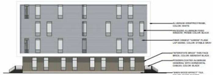
4 ELEVATION BUILDING F - EAST 3/32" = 1'-0"
