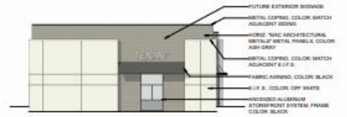
3 ELEVATION BUILDING G - SOUTH 3/32" = 1'-0"
