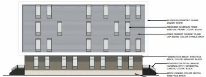
3 ELEVATION BUILDING F - WEST 3/32" = 1'-0"
