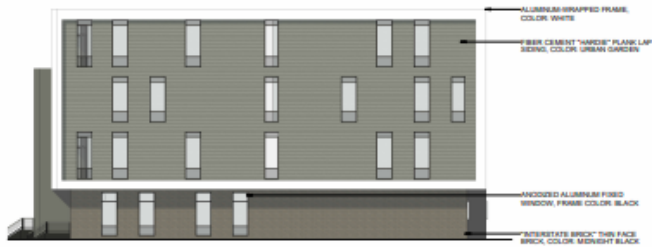
④ ELEVATION BUILDING E - SOUTH 3/32" = 1'-0"
