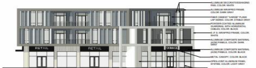
3 ELEVATION BUILDING B - NORTH 3/32" = 1'-0"
