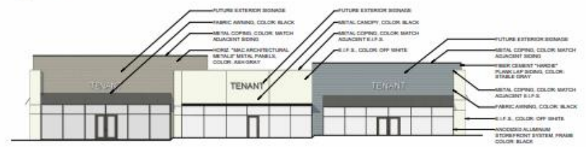
① ELEVATION BUILDING G - EAST 3/32" = 1'-0"
