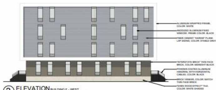
③ ELEVATION BUILDING F - WEST 3/32" = 1'-0"
