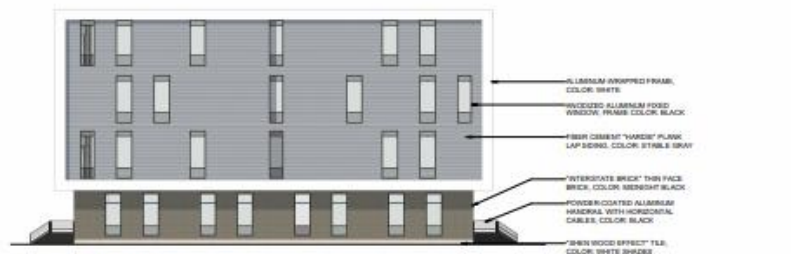
④ ELEVATION BUILDING F - EAST 3/32" = 1'-0"
